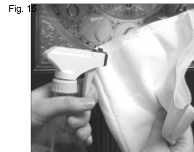
Always spray cleaning products on soft cloth, not directly on surface of clock.
